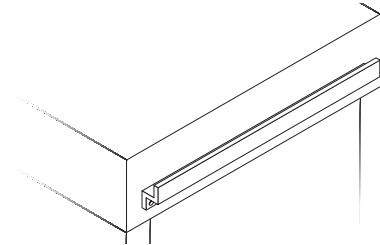
2. **Remove the floor mounting brackets from the front of the rack and insert them through the slots in the bottom front EMI bracket.**
