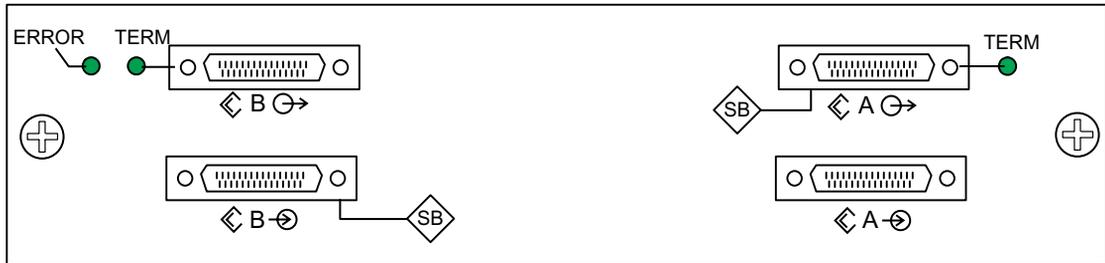
FIGURE 7-8 I/O Module for an Expansion Unit
