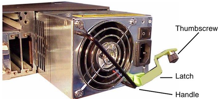
FIGURE 9-3 The Power Supply Partially Pulled out of the Chassis
