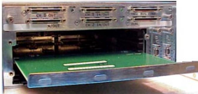
FIGURE 9-4 The Terminator Module Partially Pulled Out of the Chassis
