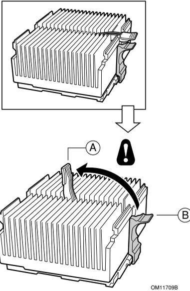
2. While depressing the black lift tab (B), press the side of the clamp opposite the lift tab towards the heatsink, then carefully lift the clamp upwards at the lift point. Once one side is unclamped, the other side can be freed by rotating the clamp bracket upwards.
