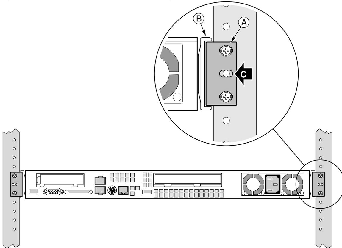
4. Slide the chassis toward the rear of the rack until the front of the chassis mounting brackets contact the front of the center posts.
