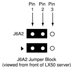
For serial devices that require a DCD signal, the J6A2 jumper block must be configured as follows: Both jumpers are in positions 2 and 3. Pin 1 is denoted by an arrow directly next to the jumper block. The following diagram provides the J6A2 jumper block pinout for this configuration.
