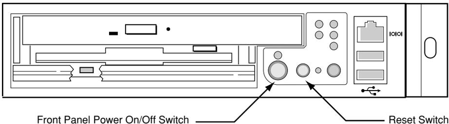
Pushing the switch sends a signal to monitoring circuitry inside the server. The switch does not directly control high-voltage AC; it controls only low-voltage signals. When the monitoring circuitry detects that the button has been depressed, it activates the power supply and powers up the server. Likewise, when the server is powered up, pushing the switch powers the server down.
