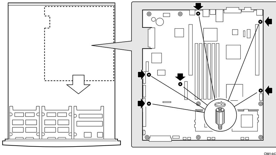
15. Slide the board toward the front of the chassis until the I/O connectors are clear of the chassis I/O openings.
