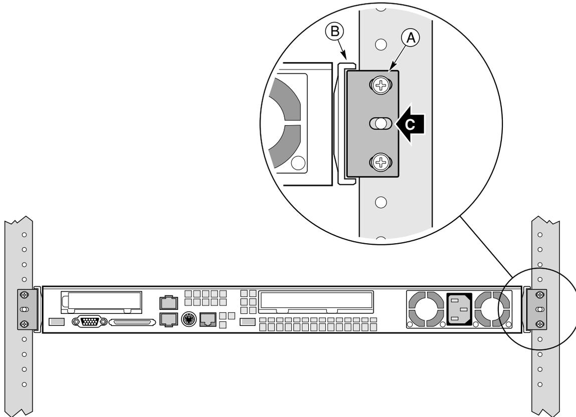
4. Slide the chassis toward the rear of the rack until the front of the chassis brackets contact the front of the center posts.
