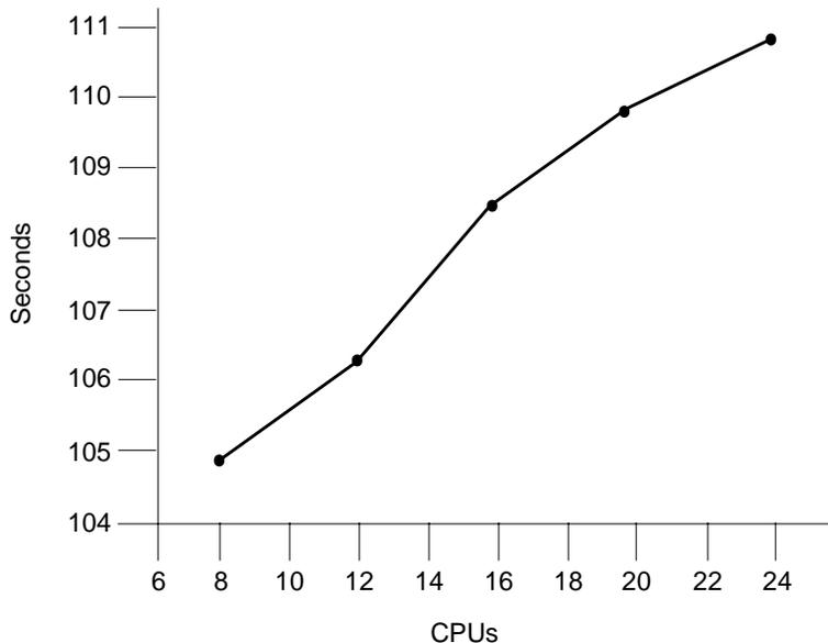
**FIGURE 7** CPUs as a Factor of the Disconnect Time
