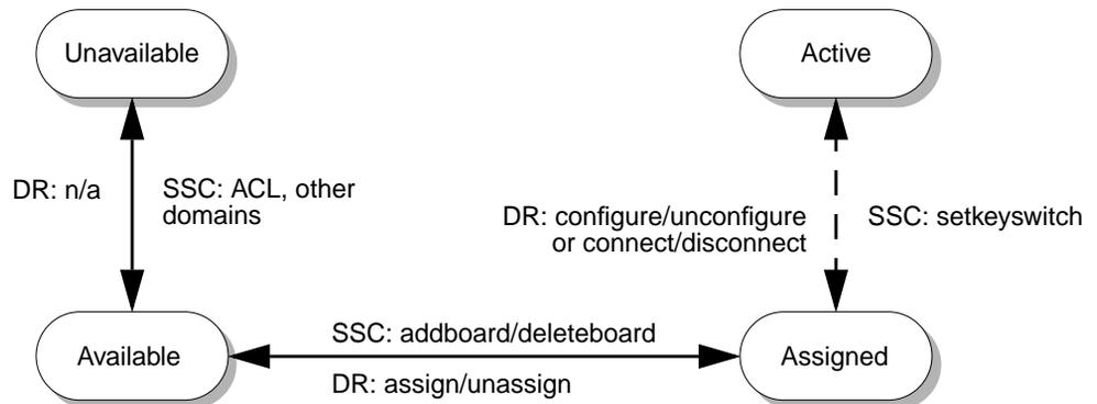
**FIGURE 1** Board States From the Perspective of the Sun Fire SSC
