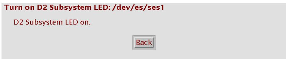
If there are no existing subsystem faults, the Subsystem LED on the front of the enclosure starts blinking amber.
