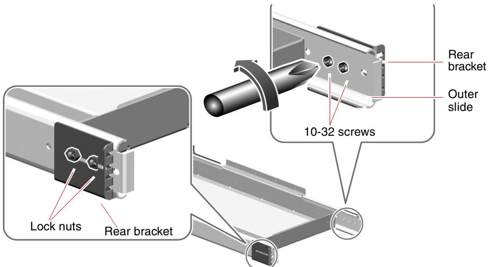
4. Attach the short rear brackets to the outer slides using two 10-32 screws and lock nuts for each short rear bracket.
