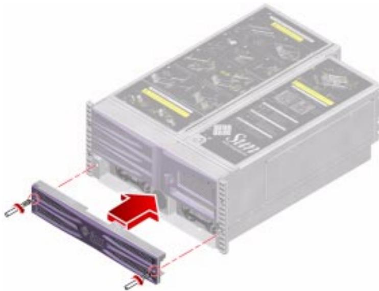
3. Using a Phillips No. 2 screwdriver, tighten the two captive screws that secure the power supply access panel to the chassis.
