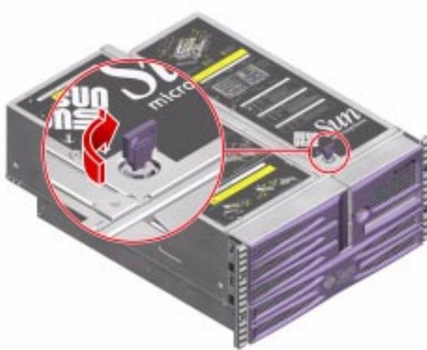
2. Loosen the three captive Phillips No. 2 screws securing the access panel to the chassis.
