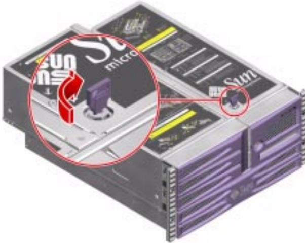
2. Loosen the five Phillips No. 2 captive screws securing the access panel to the chassis.
