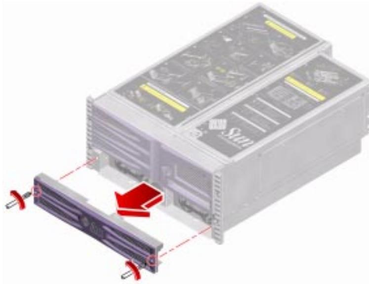
3. Pull out the power supply access panel and set it aside.
