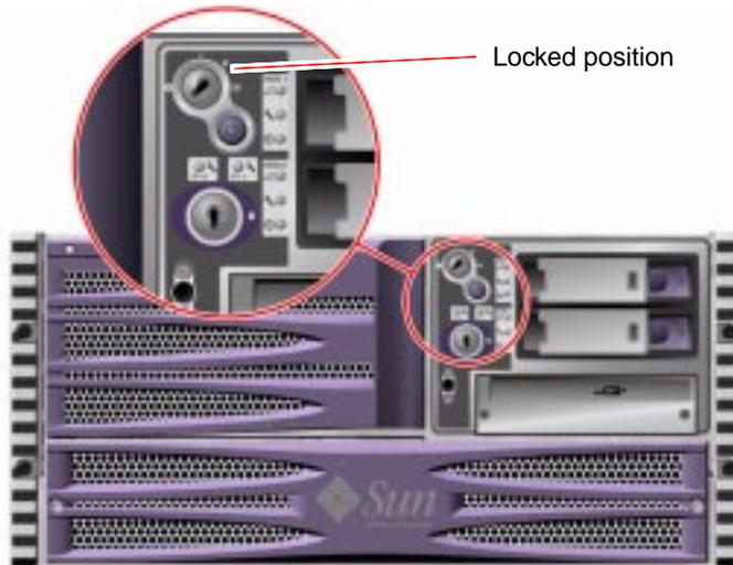
**7. Remove the system key from the system control switch and keep it in a secure place.**
