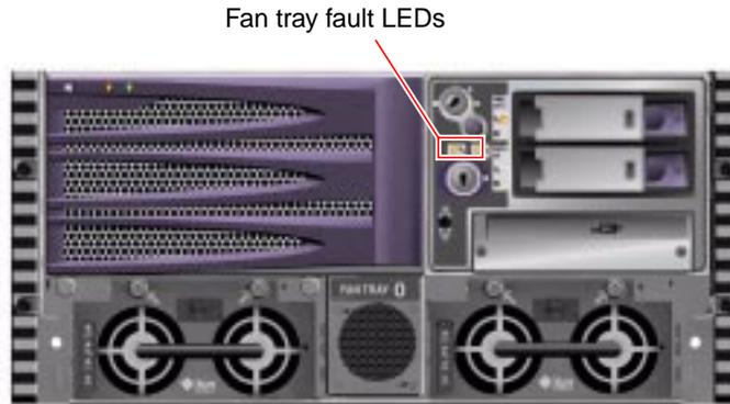
Listed from left to right, the fan tray fault LEDs operate as described in the following table.
