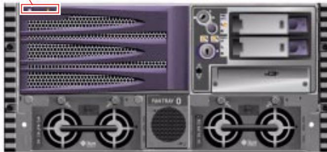
Each system status LED has a corresponding LED on the back panel.
