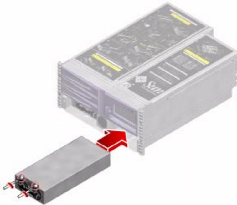
3. Push firmly on the front of the power supply to engage the connectors with the power distribution board.
