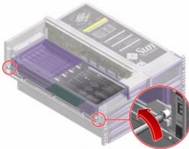
3. Rotate the CPU/Memory board ejector levers outward so that the CPU/Memory board connectors disengage from the centerplane.
