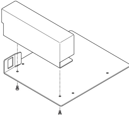
**FIGURE 4-4** Dismantling the DAT Filler Panel
