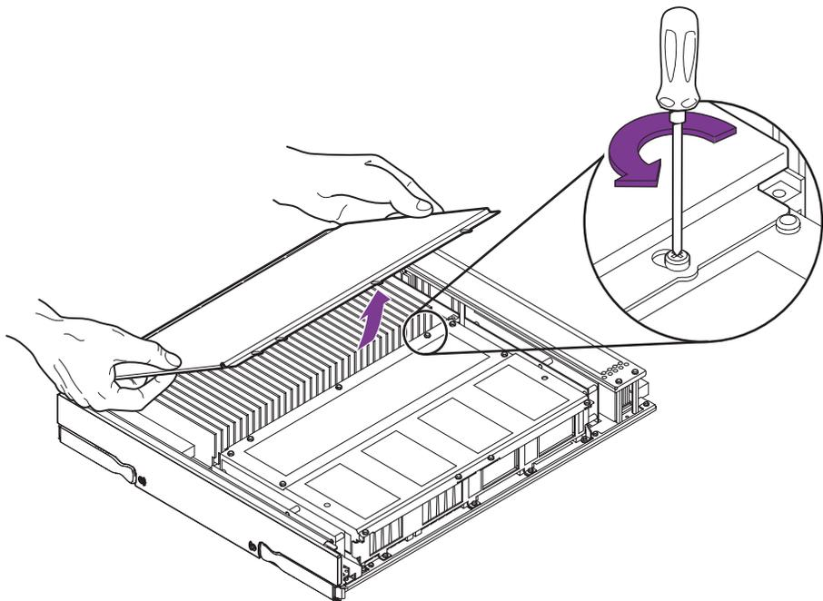
**FIGURE 7-6** Removing the DIMM Cover
