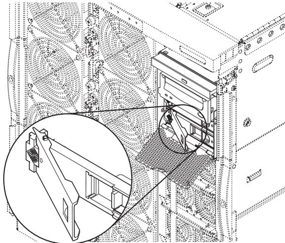
**FIGURE 4-2** Ejecting the Hard Disk Drive
