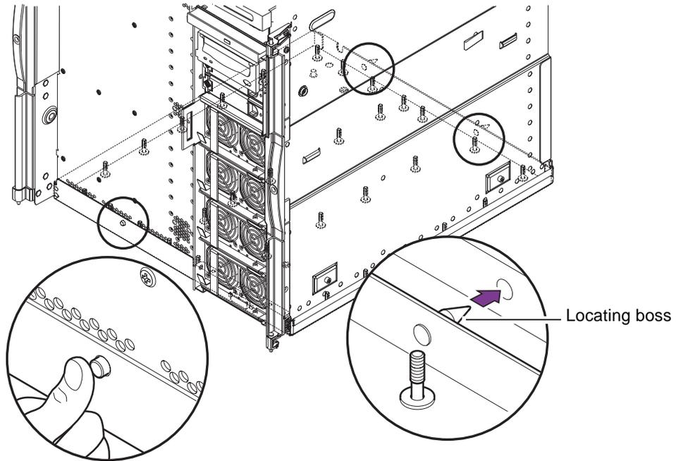
FIGURE 11-2 Releasing the Baseplane Securing Button
