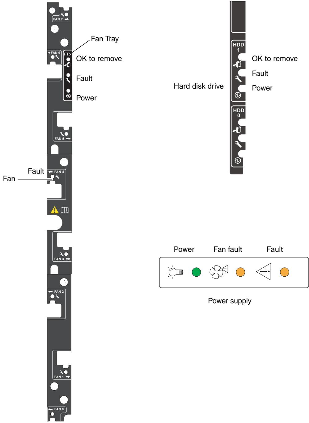
**FIGURE 1-9** Power Supply, Hard Disk Drive, Fan and Fan Tray Indicator LEDs
