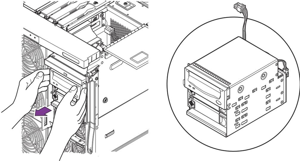
FIGURE 4-14 Removing the Media Bay
