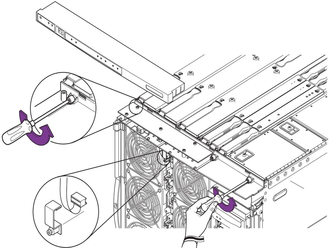
**FIGURE 10-2** Removing the System Indicator Board Connector and Securing Screws
