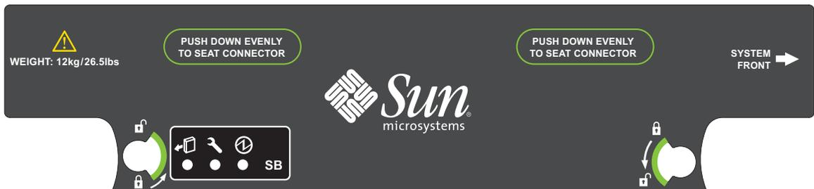
FIGURE 7-1 CPU/Memory board Labels and Indications
