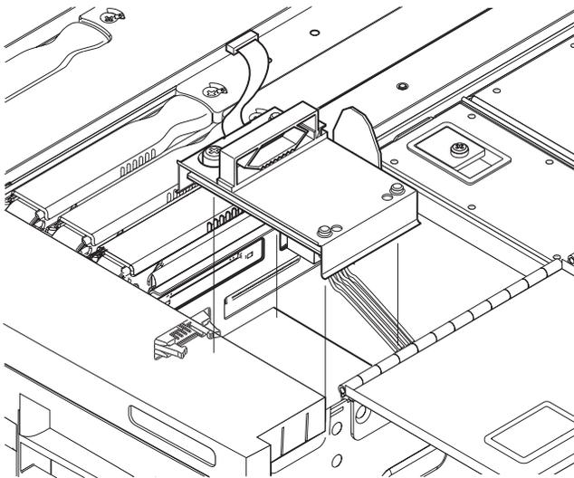
**FIGURE 4-10** Removing the SCC Reader
