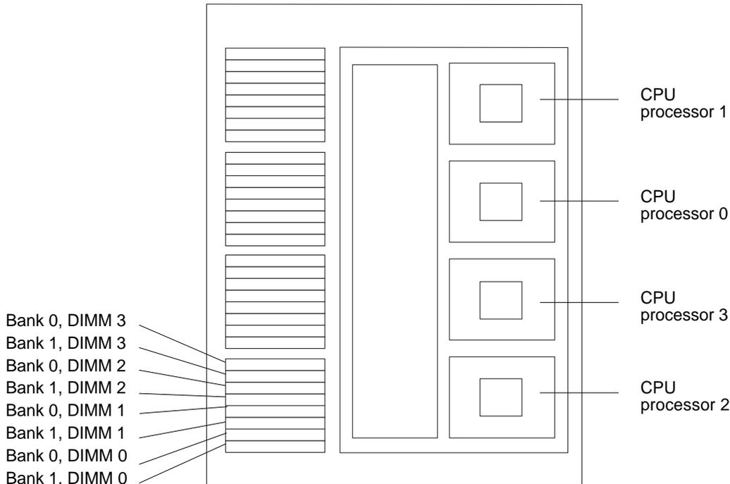
**FIGURE 7-5** DIMM Slot Numbers
