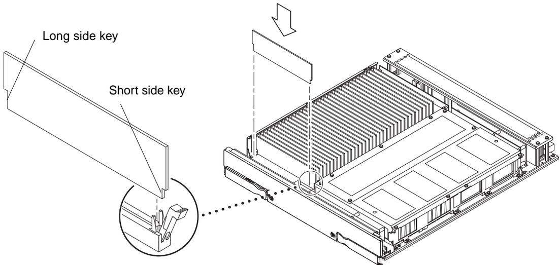
**FIGURE 7-8** Installing a DIMM
