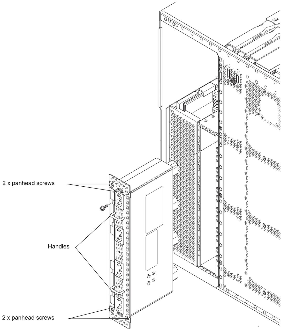
**FIGURE 6-3** Removing the Power Inlet Box
