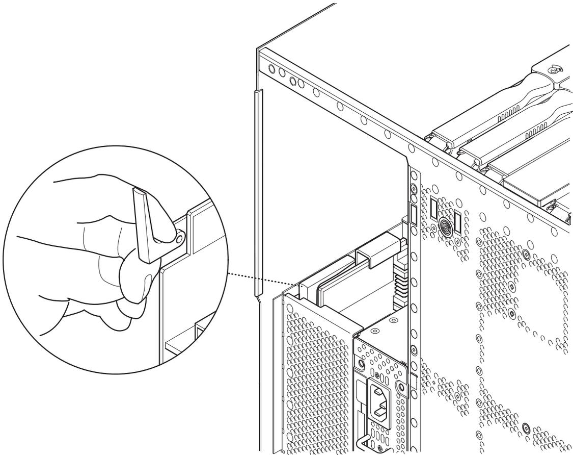
**FIGURE 6-4** Disengaging the PDB Ejector Lever
