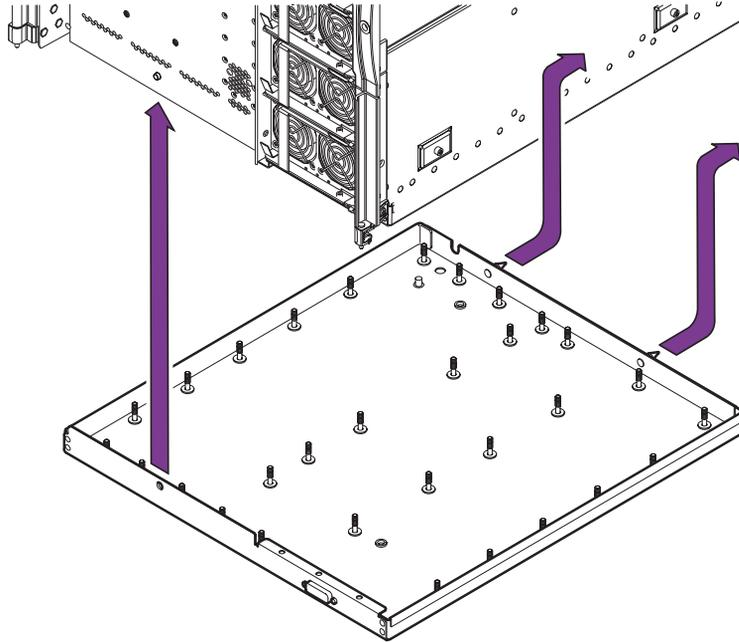
FIGURE 11-3 Removing the Baseplane
