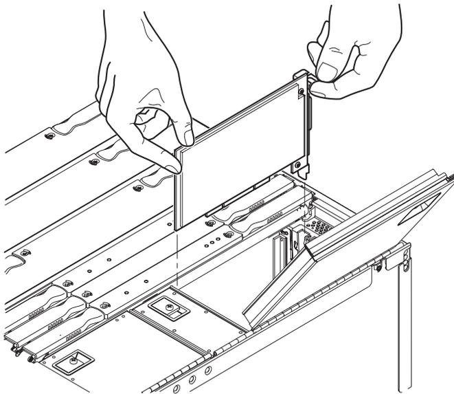
**FIGURE 8-6** Removing a PCI Card
