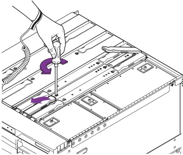
**FIGURE 9-1** Unlocking the L2 Repeater Board Ejector Levers
