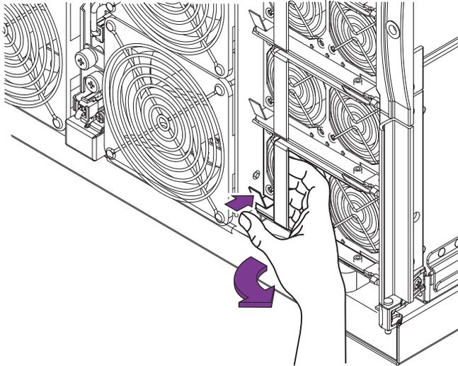
**FIGURE 6-1** Unlatching a Power Supply
