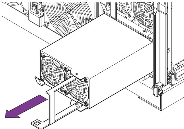
**FIGURE 6-2** Removing the Power Supply
