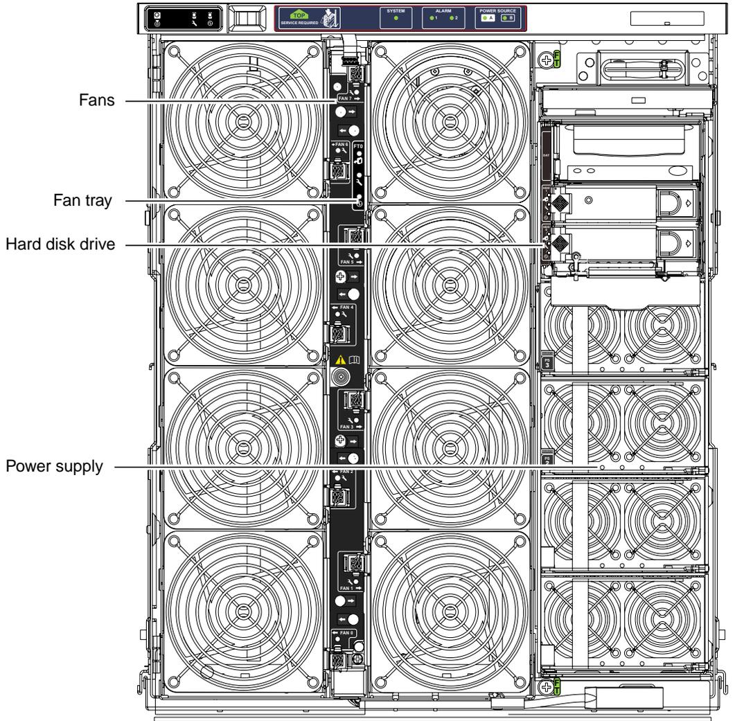
**FIGURE 1-8** Module Indicator LED Locations – Front of System
