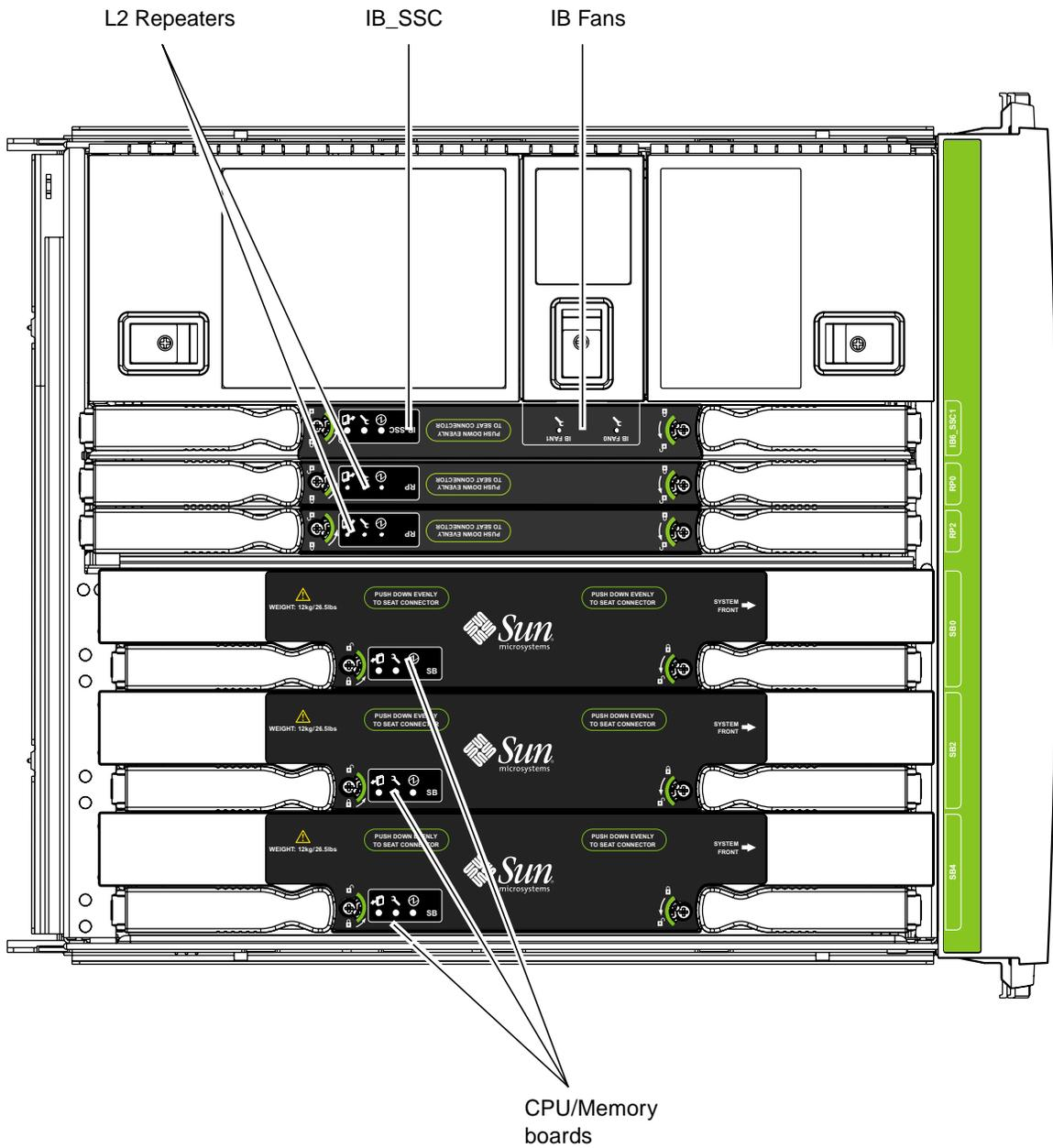
FIGURE 1-4 Locations of Modules and Indicator LEDs – Top of System
