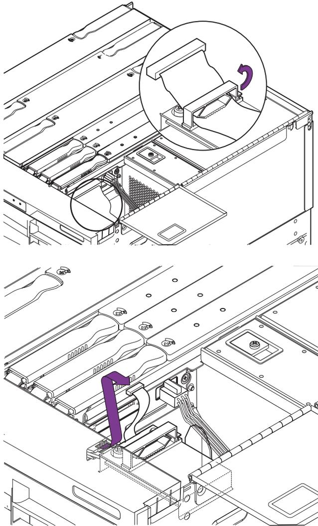
**FIGURE 4-8** Disconnecting the SCCR Cables
