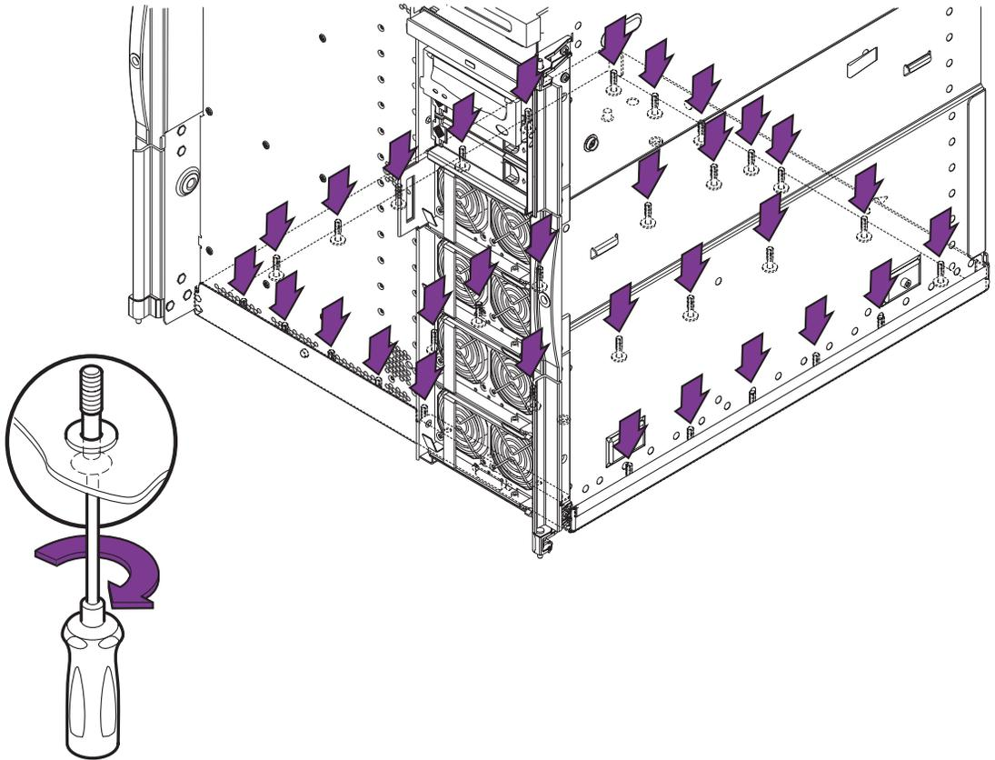
**FIGURE 11-1** Removing the 31 Baseplane Securing Screws
