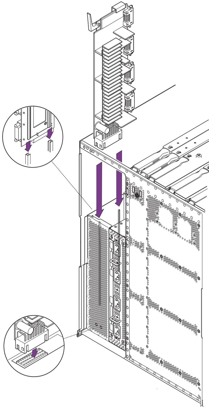
FIGURE 6-6 Inserting the PDB
