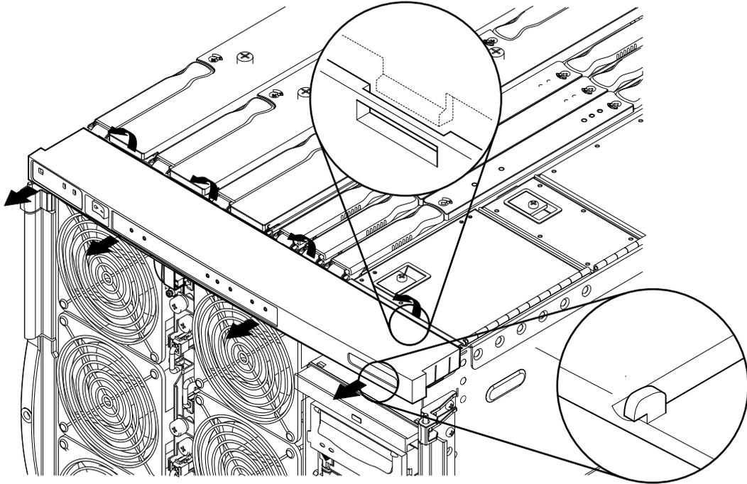
FIGURE 10-1 Removing the System Indicator Board Cover
