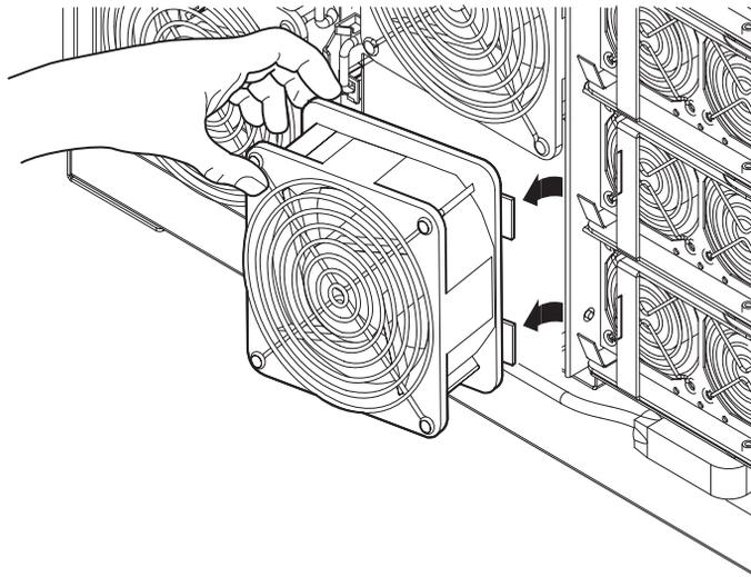
**FIGURE 5-3** Removing a Fan
