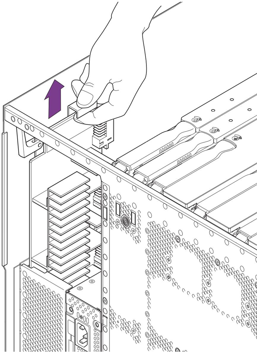
FIGURE 6-5 Removing the PDB
