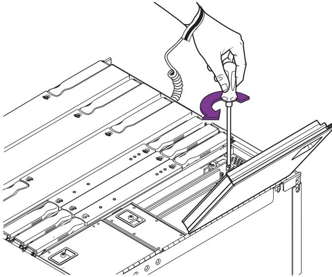
**FIGURE 8-5** Removing the PCI Card Retaining Screw
