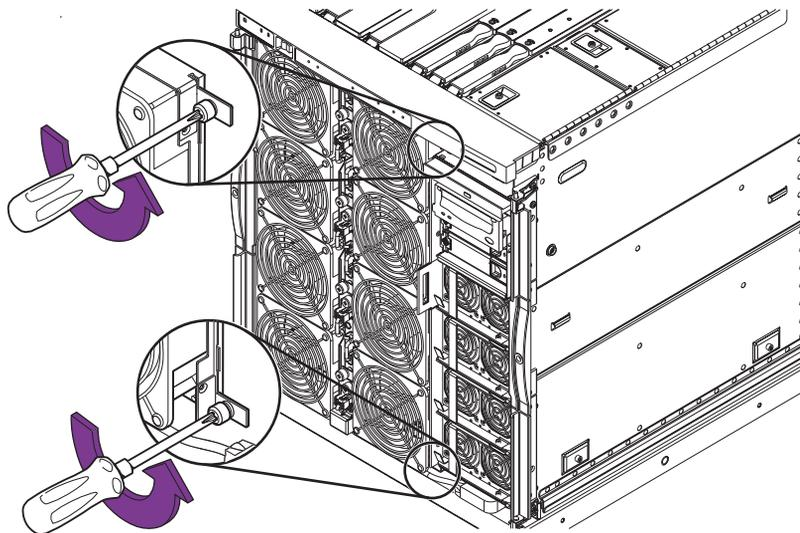
**FIGURE 5-5** Loosening the Fan Tray Retaining Screws
