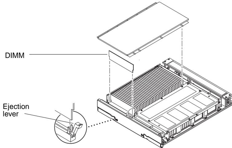
FIGURE 7-7 Removing a DIMM
