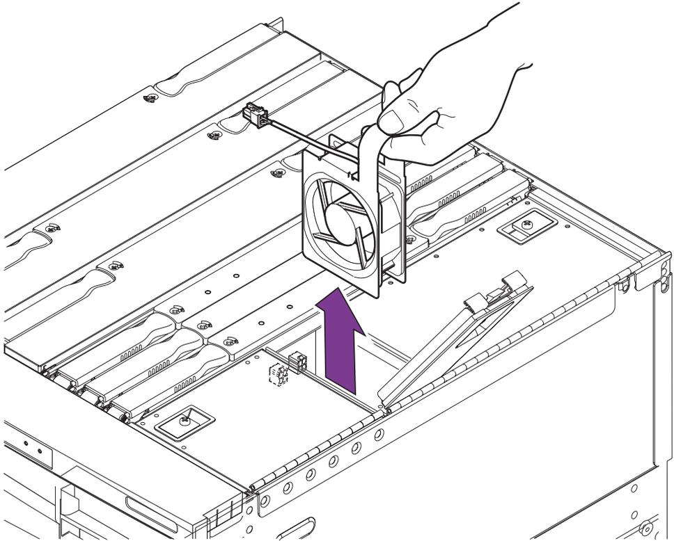
**FIGURE 5-9** Removing an IB\_SSC Fan
