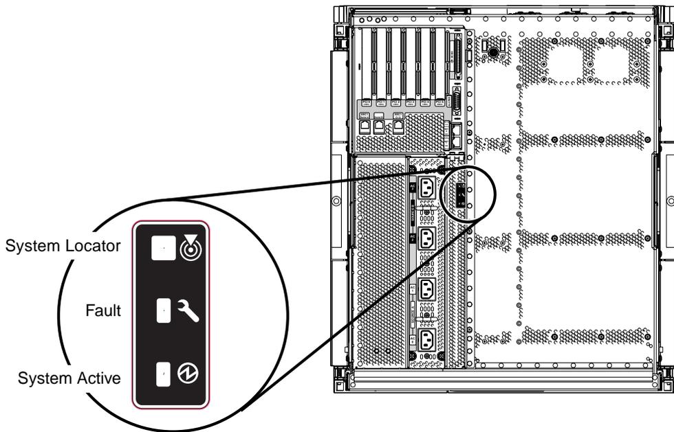
**FIGURE 1-3** Enclosure Level System Indicator LED Repeater on the Back Panel
