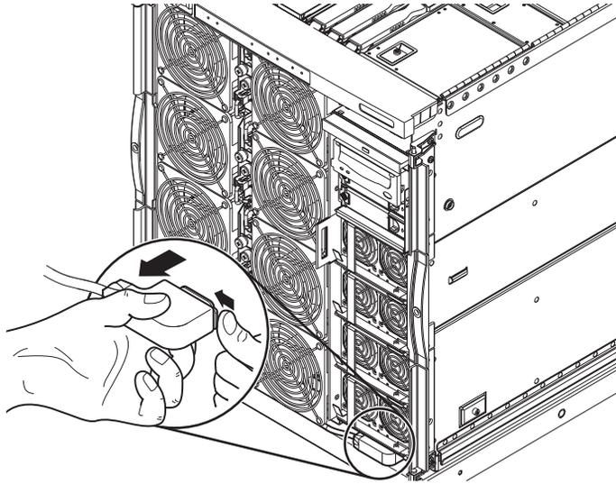
**FIGURE 5-4** Removing the Fan Tray Power Connector
