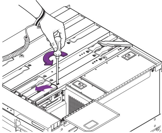
**FIGURE 8-2** Unlocking the IB\_SSC Assembly Ejector Levers
