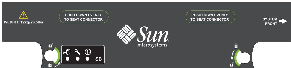
FIGURE 1-5 CPU/Memory board Indicator LEDs
