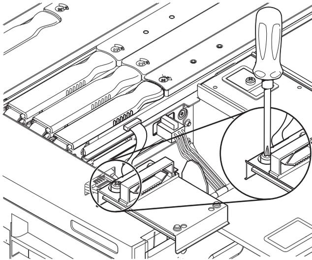
**FIGURE 4-9** Loosening the SCC Reader Captive Screw
