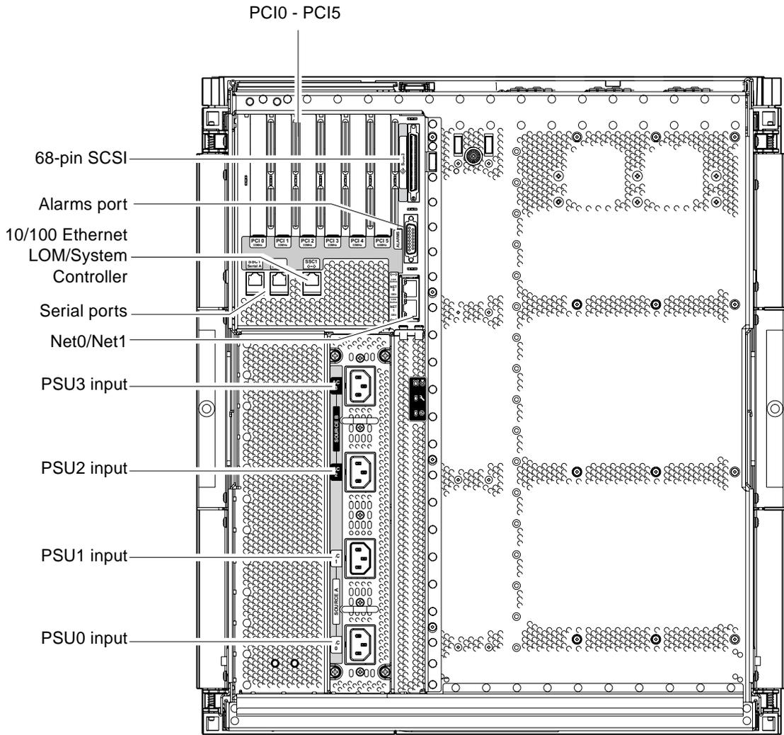
FIGURE B-1 External I/O Connections
