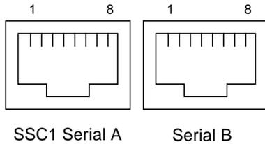
**FIGURE B-3** RJ45 Serial Connectors
