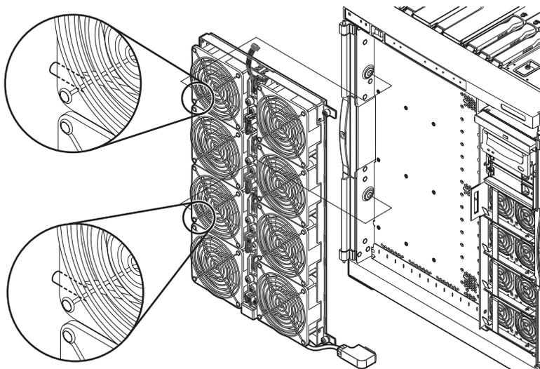
**FIGURE 5-6** Removing the Fan Tray
