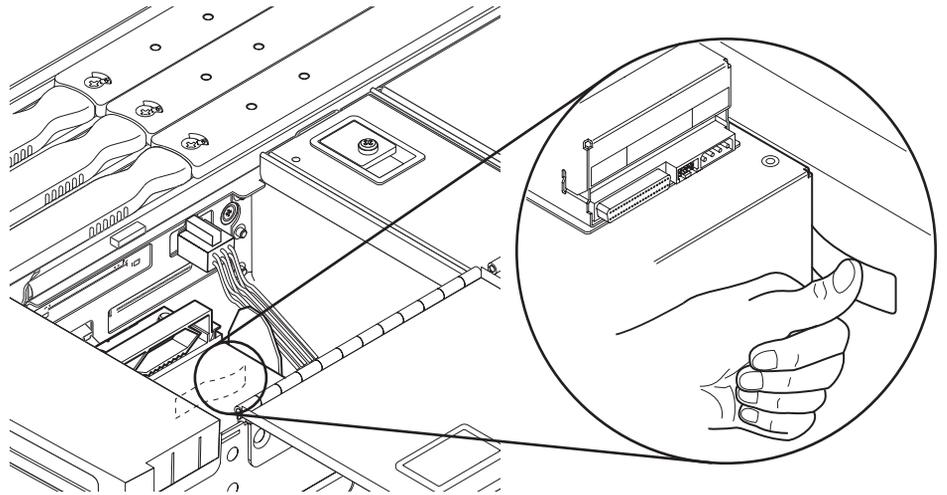
FIGURE 4-12 Releasing the Media Bay Retaining Spring
