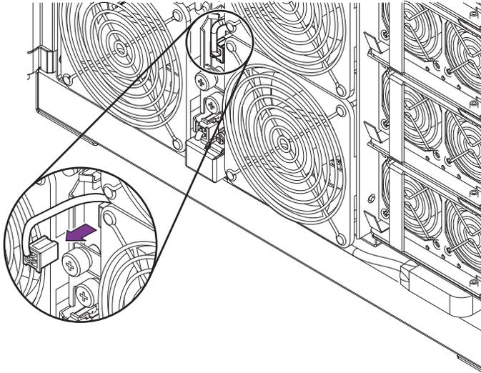
**FIGURE 5-1** Unplugging the Fan Power Connector
