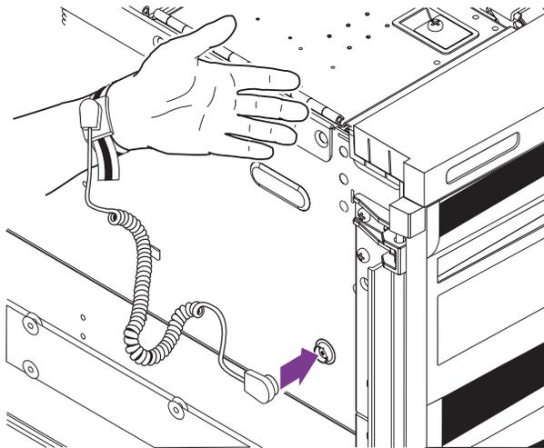
**FIGURE 2-2** Attaching the Antistatic Wrist Strap – Left-Hand Side
