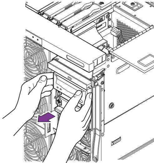
FIGURE 4-13 Pulling Out the Media Bay a Short Distance
