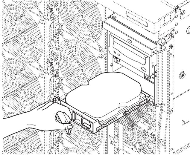
**FIGURE 4-3** Removing the Hard Disk Drive
