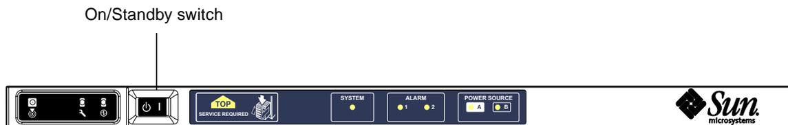
FIGURE 3-1 Sun Fire V1280 Server Power (On/Standby) Switch04
