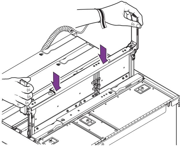
**FIGURE 9-3** Inserting an L2 Repeater Board
