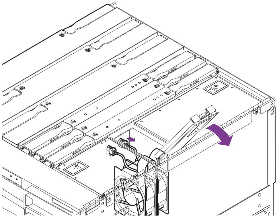
**FIGURE 5-8** Identifying the Fan Connector
