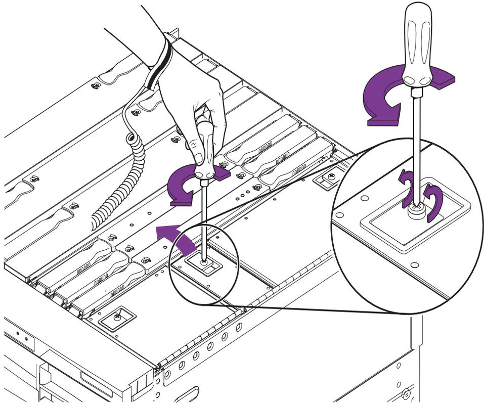
**FIGURE 5-7** Opening the IB Fan Cover
