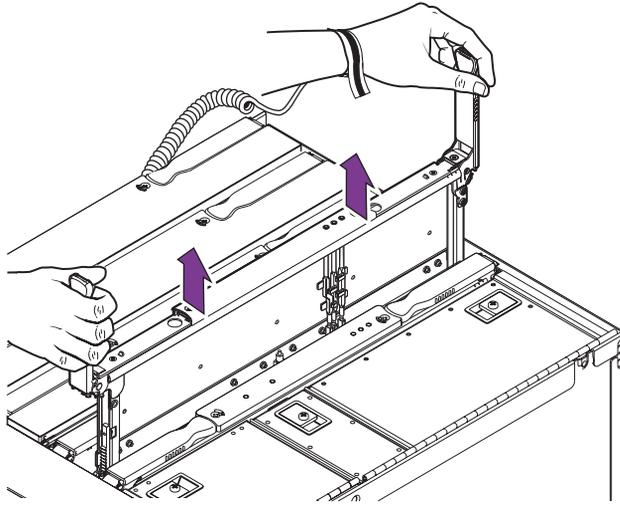
FIGURE 9-2 Raising an L2 Repeater Board
