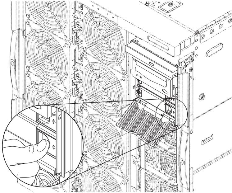
**FIGURE 4-1** Releasing the Hard Disk Drive Ejector
