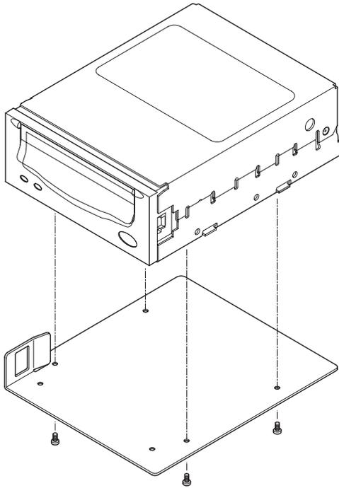
**FIGURE 4-5** Assembling the DAT drive
