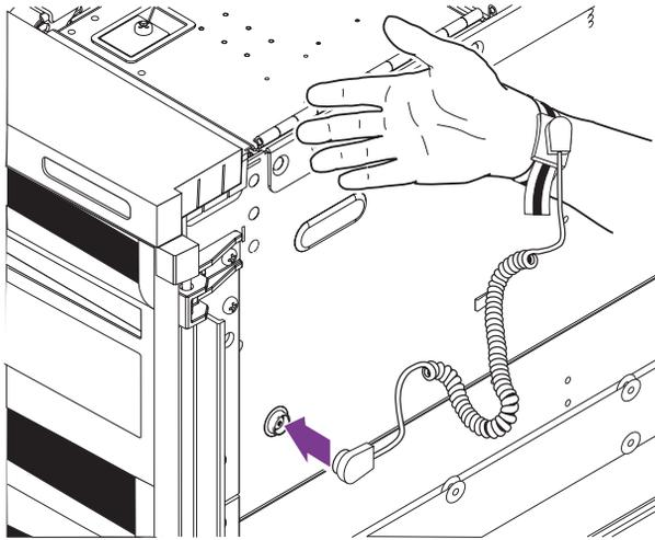
**FIGURE 2-1** Attaching the Antistatic Wrist Strap – Right-Hand Side
