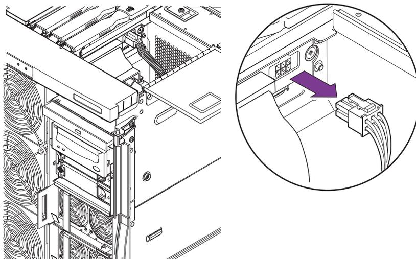
**FIGURE 4-11** Removing Cables from the IB\_SSC Assembly to the Media Bay
