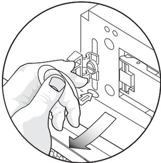
FIGURE 5-11 Pulling the Head of the Tether Entirely Out of the Chassis
