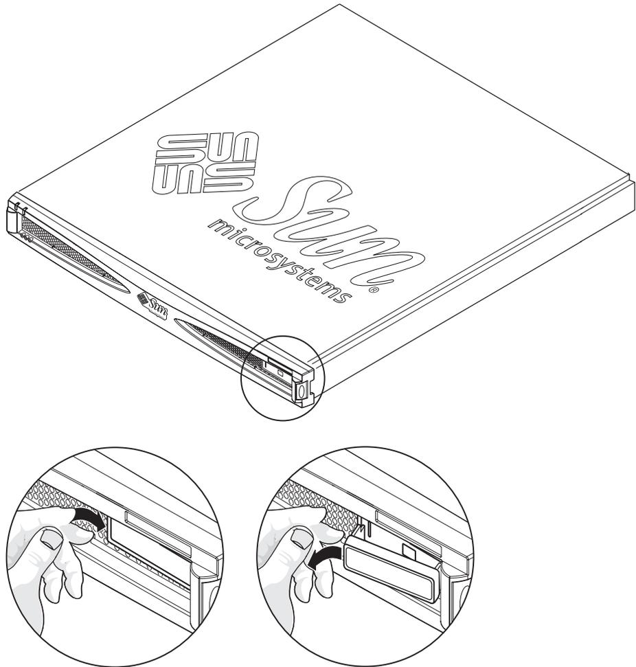
**FIGURE 1-4** Releasing the Left Retaining Lug to Make the Nameplate Swing Out
