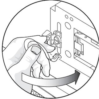
FIGURE 5-10 Pushing the Tether In the Opposite Direction
